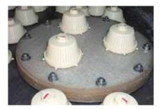
Internal Nozzle Plate Service Hatch
