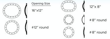
Waterco's advanced manufacturing capabilities have enabled it to incorporate sight glasses and large manholes into its high-pressure fiberglass filters. Waterco Micron Side Mount Deep Bed Commercial filters are available with the option of:
