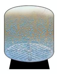
Conventional laterals are not suitable for large-scale commercial filters as "dead legs" exist between the laterals, which compromises water flow through the filter bed. Waterco's unique "fish tail" or "fish bone" lateral configuration eliminates this problem by providing effective coverage of the filter bed and balanced water flow.
